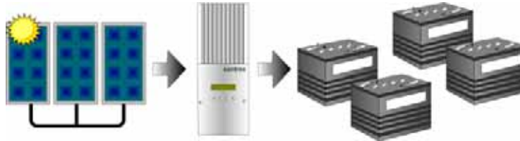
Figure 1-3 PV Charge Controller
